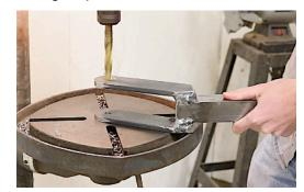
Drill and tap a ring of four holes in the right fork side to accept the 1/4"-20 bolts that will hold the tracking adjustment flange in place. These holes need to align very closely with the 5/16" holes in the flange, and if you are concerned that you may not be able to make them line up well 1/2" hole in left side 9/16" hole in right side
