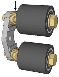
and put a belt loosely in place. Slip the belt deflector on from the front, and attach it to the middle hole in the small wheel holder using a 3/8"-16 x 1-1/4" bolt. Now you can re-install the small wheel by slipping it behind the belt and into the holder. I recommend watching my video for clarification if this doesn't make sense.
