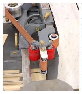
The belt deflector can be installed on either the left or right side of the small wheel holder, and the boomerang can face forward or backward. To install it, first remove the small wheel from the holder,
