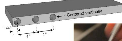
caliper to scribe lines for where the holes would be drilled, then carefully center-punched them and drilled them with a drill press. They need to be drilled deep enough that you can tap a clean thread 3/8" to 1/2" deep, but avoid drilling excessively deep as that will weaken the plate too much.
