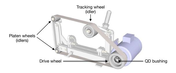
**Bearings** The bearings I used are Timken P203PP, 17mm ID, 40mm OD, 12mm width, double sealed. This is a very common size of bearing. They are rated for a max RPM of 11,050, which is important since the platen wheels will spin 2.5x as fast as the motor.
