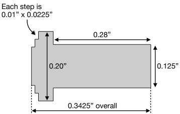
I made this part by modifying a button head screw, but figured I'd include it anyway. The shape of the head was just eyeballed to look nice.
